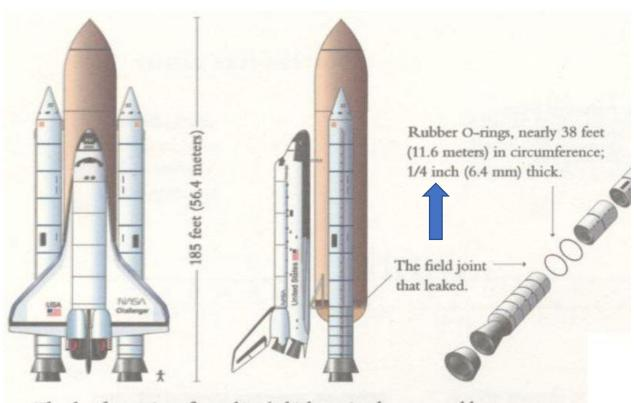
The shuttle consists of an *orbiter* (which carries the crew and has powerful engines in the back), a large liquid-fuel *tank* for the orbiter engines, and 2 solid-fuel *booster rockets* mounted on the sides of the central tank.
